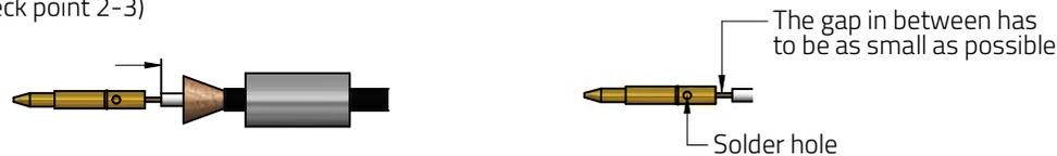
**Step 4.** Push cable with center contact into connector main body until perceptive point. Cover cable braid over connector neck carefully
